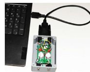
This is the configuration for the DB-9 to USB Connector showing DB-9 connected to the Interface and the USB connected to a Laptop Computer
